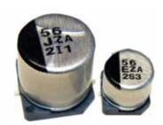
Type HZA hybrid capacitors are a combination of solid polymer aluminum technology with wet aluminum electrolytic technology. This results in a surface mount capacitor with a 10,000 hour life, low leakage current, high voltage capability, very low esr and small case sizes. They are ideal for high density PC board designs. The vertical cylindrical cases facilitate automatic mounting and feature high reflow soldering temperature capability. Type HZA is RoHS compliant.
